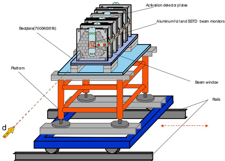
◆ - Displacement of SSTD and threshold activation detectors on surface of "Quinta" setup
